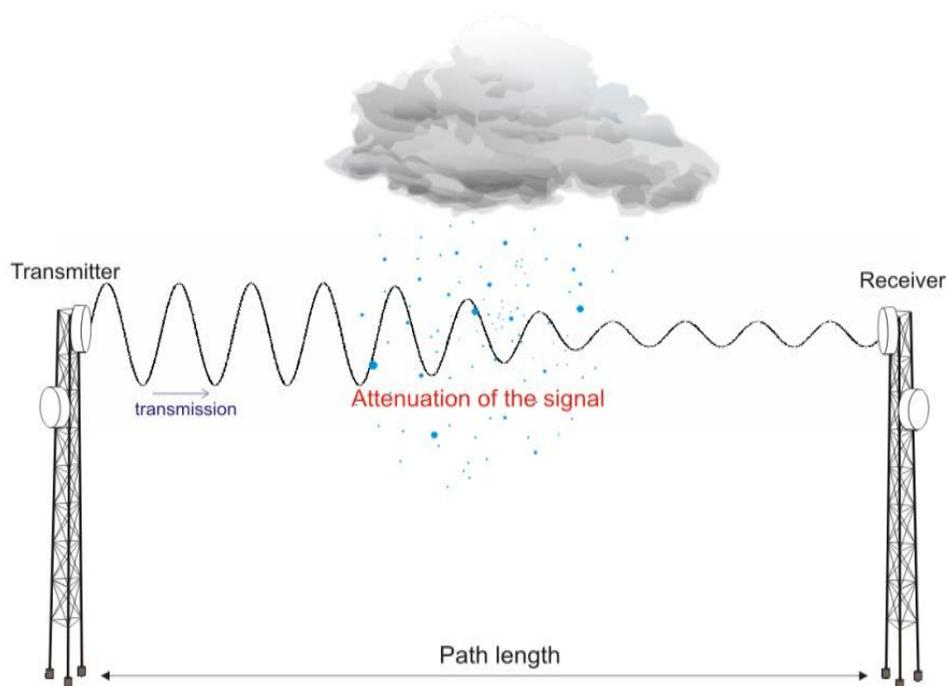
**Figure 1: Shows a schematic microwave link and attenuation of the signal.**
