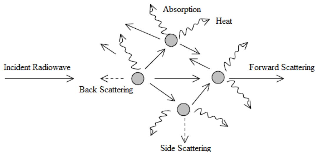
**Figure 2: shows Interaction of an incident radio wave with rain drops.**
