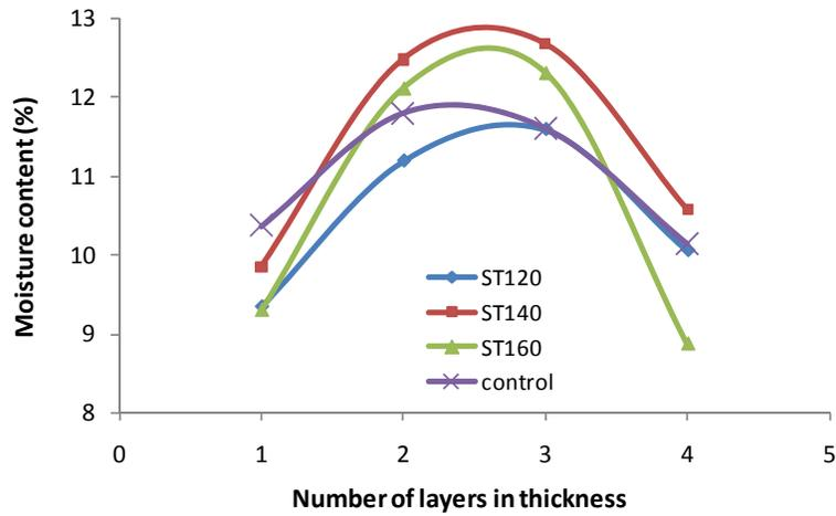
**Fig. 5.** Moisture content gradient in steam exposed fir wood specimens compared to the unexposed ones
