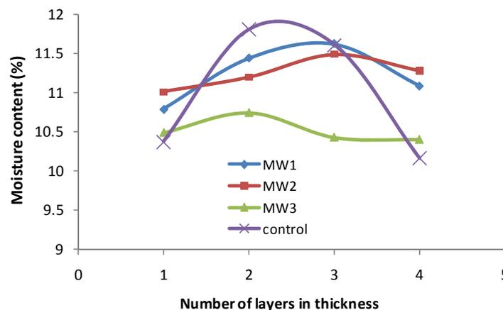
**Fig. 4.** Moisture content gradient in microwave exposed fir wood specimens compared to the unexposed ones
