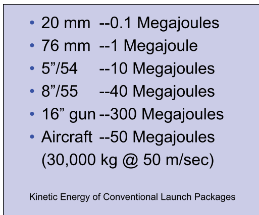
Figure 6. Launch Energy of Various Projectiles
